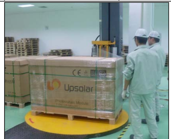
Step four: Each finished pallet is wrapped in plastic film to ensure pallet integrity
