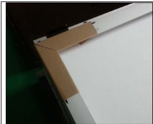
Step one: Four paper corners are fixed to each frame to avoid any contact
