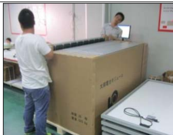
Step two: Twenty-six modules are vertically placed into the carton for each pallet
