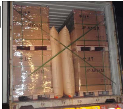
Each finished pallet is wrapped in plastic film to ensure the pallet integrity
